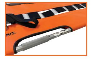
Depress the button (detent) that keeps the knurled locking tube in the storage position. Slide the knurled tube over the hinge until the button (detent) snaps up and locks the knurled tube over the hinge. Make sure that both hinges are stabilized by the knurled locking tubes. This makes the Stretcher ridged and ready for use.
