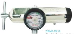
Click-Style Regulator with Hose Barb Outlet, two DISS Outlets and CGA 870 Yoke Inlet
