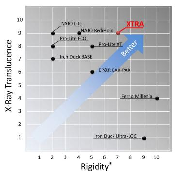
\*Rigidity specification based upon the deflection from horizontal of the center of the backboard with a 400 lb. distributed load, backboard supported at each end.
